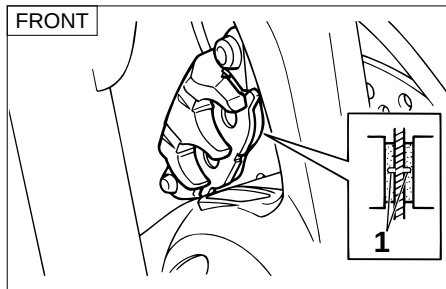
1. Wear indicator groove
